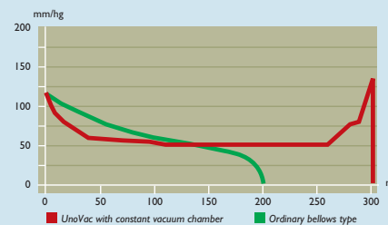
UnoVac provides a constant suction level in comparison with traditional bellows-type units.
